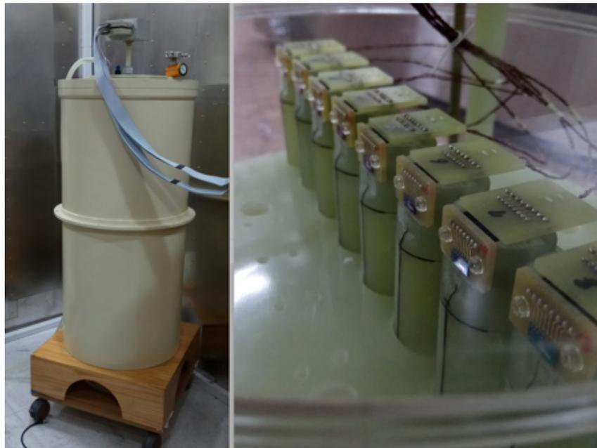
**Fig. B.5:** Time-averaging measurements were made with a set-up having the same electronics but different designs of the (left) dewar and (right) gradiometer [2]. The figure is licensed under [CC-BY-4.0](https://creativecommons.org/licenses/by/4.0/).
